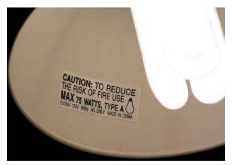
The adjoining picture shows the interior of a lightsocket. The socket's maximum rating, for incandescent bulbs, is 75 Watts. However, the socket contains a CFL, rather than an incandescent bulb.
